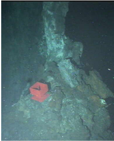
Fig. 14.1. Magnetic collector, “near” deployment. Left “Near” collector deployed 3 m away from a black smoker chimney at Bio9 vent. Right Four magnets within the “near” collector, covered with particulates after 19 days of deployment. (Alvin Dive #4294).
