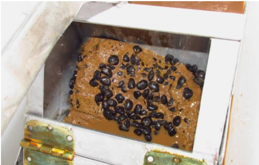
Figure 22. Rounded pebbles of volcanic rock coated with a chilled margin of volcanic glass. Collected from the subducting plate in RG #10.
