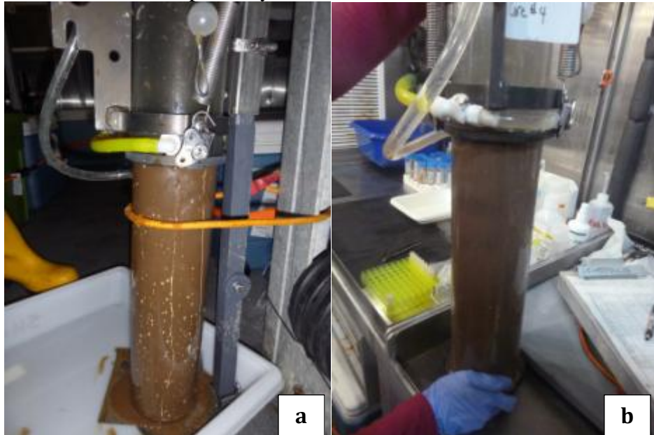
Figure 4. Sediment core recovered by the FVCR at the CR05 site at 7942 meters.
