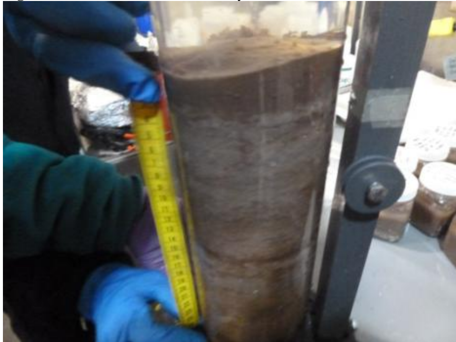
Figure 4. Sediment core recovered by the FVCR at the CR05 site at 7942 meters.
