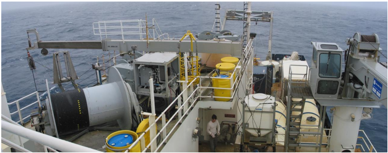
Fig. 1. MULVFS shown deployed from the starboard side of R/V Revelle. Shown are the drum winch and associated hydraulic power system, level wind, electromechanical and wire handling system. Photo from 2002 during the Southern Ocean Iron Experiment. Setup during VERTIGO was identical.
