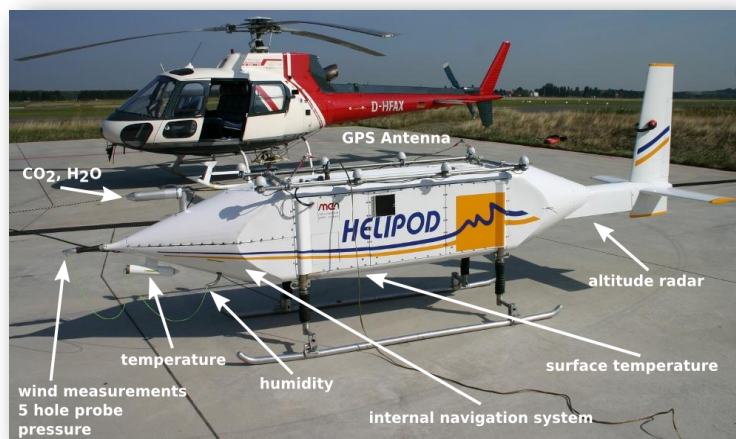
Fig. 3.2: The Helipod and its instrumentation
