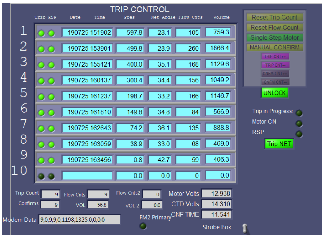
Figure 2. Nets depths, angle, flow counts and volume for the MOCNESS tow. Volumes seemed too high for the towing conditions. Corrections were made for the processed data files.
