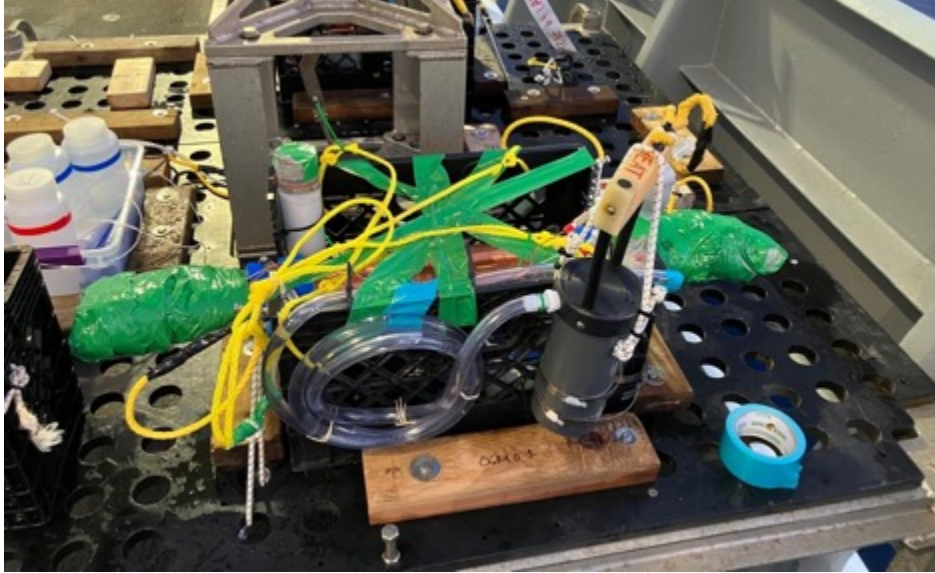
Figure 18. View of the assembled Green OsmoSampler attached to the elevator. Wooden blocks were used to create a cradle for the milkcrate, with bungee cord tie points on either of the shorter sides of the milkcrate. Prior to elevator deployment, the intakes of the OsmoSamplers were connected to syringes filled with ultrapure water; these were removed immediately prior to deployment.
