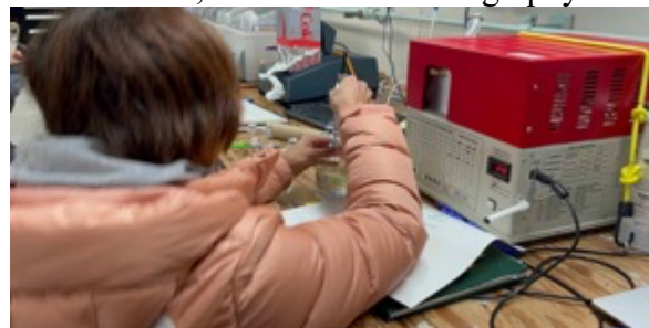
Figure 11 Shipboard GC analysis of extracted \text{CH}_4 concentration in a serum bottle.
