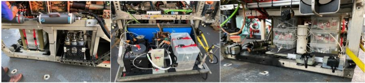
Figure 4. Third party equipment on Jason for dive J2-1509: The starboard swing arm (left), front porch (middle) and aft (right).
